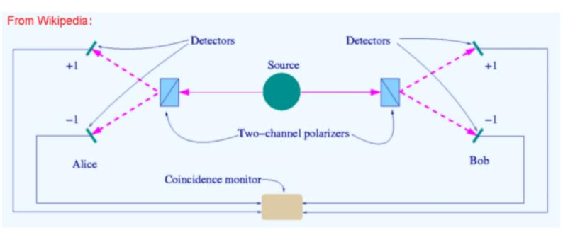
The source sends pairs of "photons", one in each direction.
